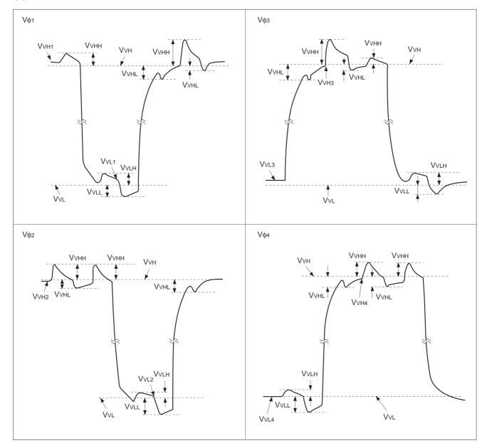
$$\begin{split} V_{VH} &= (V_{VH1} + V_{VH2})/2\\ V_{VL} &= (V_{VL3} + V_{VL4})/2\\ V_{\varphi V} &= V_{VHN} - V_{VLN} \ (n=1 \ to \ 4) \end{split}$$
