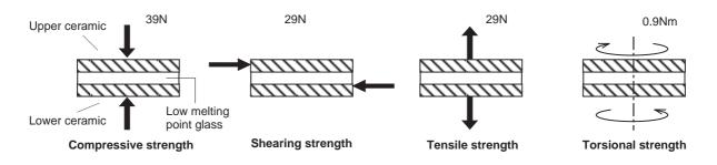
b) If a load is applied to the entire surface by a hard component, bending stress may be generated and the package may fracture, etc., depending on the flatness of the ceramic portions. Therefore, for installation, use either an elastic load, such as a spring plate, or an adhesive.
