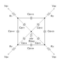
Vertical transfer clock equivalent circuit
