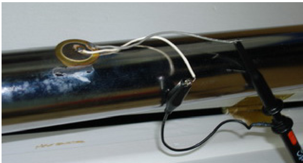
Figure 2 Piezoelectric sensor attached to leg
