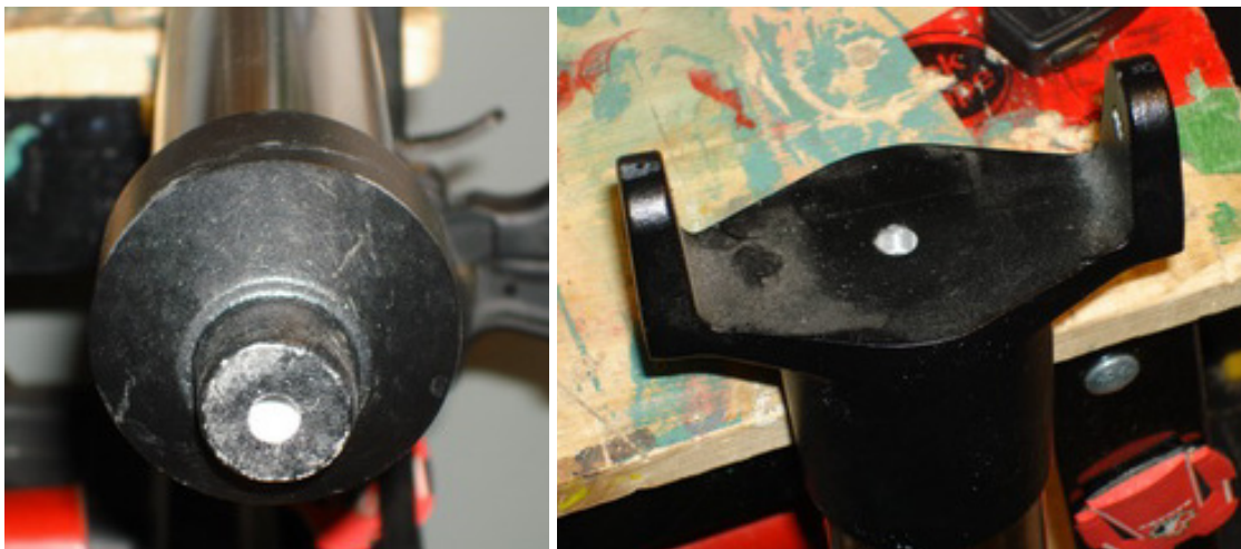
Figure 4 Holes drilled in either end of leg
