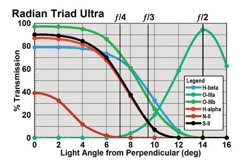
Figure 11 - Theoretical Radian Triad Ultra Nebula Wavelength Transmission vs Angle
