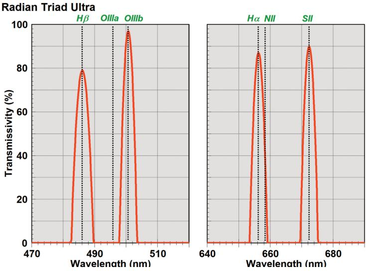
Figure 10 - Theoretical Radian Triad Ultra Spectral Transmissivity
