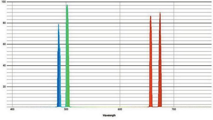
Figure 2 - OPT Radian Triad Ultra Spectral Response (courtesy OPTCorp)
