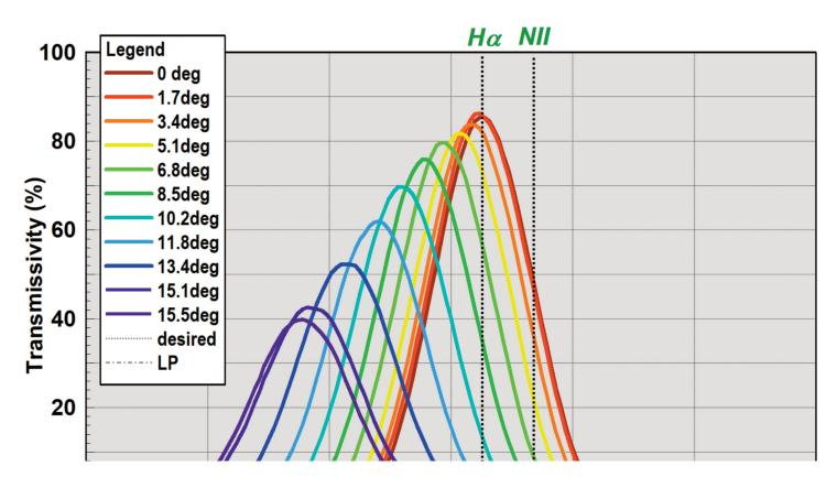
Figure 5 Measured Radian Triad Spectral Response vs Angle - Halpha Pass Band
