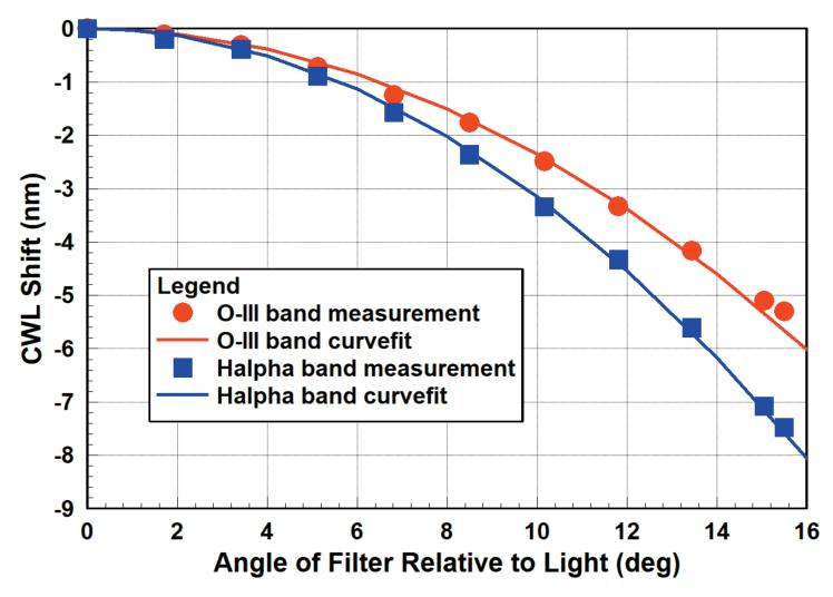
Figure 6 - Measured Radian Triad CWL Shift vs Angle
