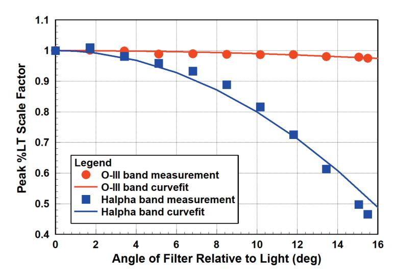
Figure 8 - Measured Radian Triad Peak %LT Scale Factor vs Angle
