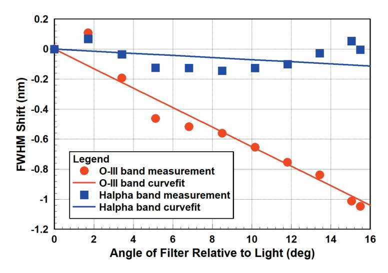
Figure 7 - Measured Radian Triad FWHM Shift vs Angle
