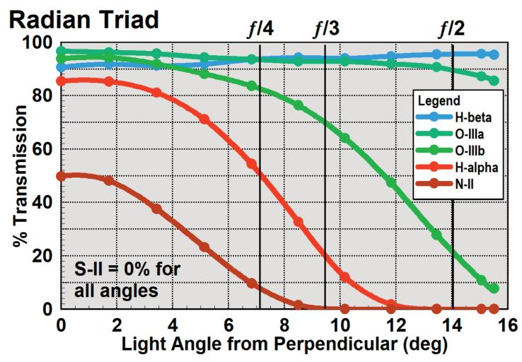
Figure 9 - Measured Radian Triad Nebula Wavelength Transmission vs Angle
