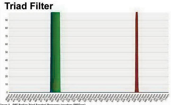
Figure 1 - OPT Radian Triad Spectral Response (courtesy OPTCorp)
