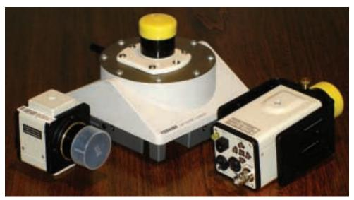
Figure 4. Author's Astro-Video Cameras: The author owns three cameras for video astronomy (from left): Mallincam Junior, Toshiba IK-WB11A net-cam, and Mallincam Xtreme.
