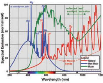
Figure 4. Absolute LP and DSO Emissions: These spectral emissions are to scale, allowing for them to be added together and compared with and without filters.
