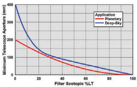
Figure 6. Recommended Minimum Percentage LT Versus Aperture: All filters reduce the amount of light getting to the eye. It is important to pick a filter that is not too dark for your aperture.
