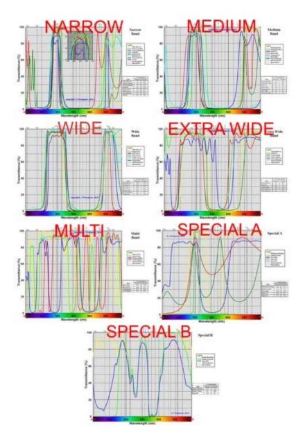
Figure 13 Deep-Sky Filter Spectral Response Comparison Plots
