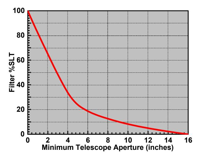
Figure 3 Minimum Recommended Telescope Aperture For Visual Observation
