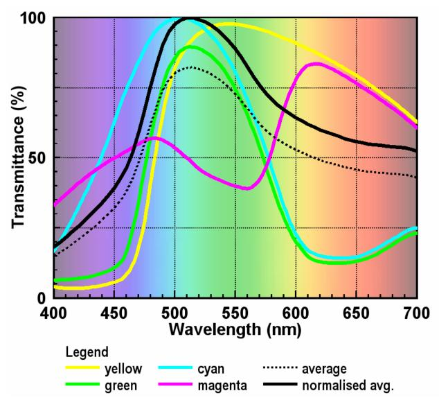
Figure 1 Spectral Response Of The Sony ICX418AKL-A CCD
