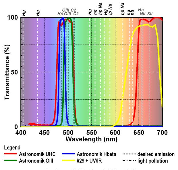
Figure 5 Band-Pass Filters Used In Test – Part 2
