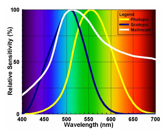
Figure 2 Relative Spectral Response - Human Eye vs. Mallincam
