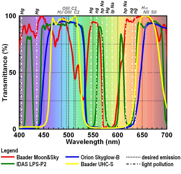
Figure 4 Band-Pass Filters Used In Test - Part 1
