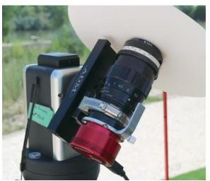
Figure 3: Eclipse day image of lens, camera, and filters on Cube Pro mount. (image by J. Thompson)
