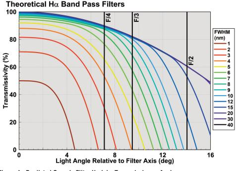
Figure 4 - Predicted Generic Filter H-alpha Transmission vs Angle
