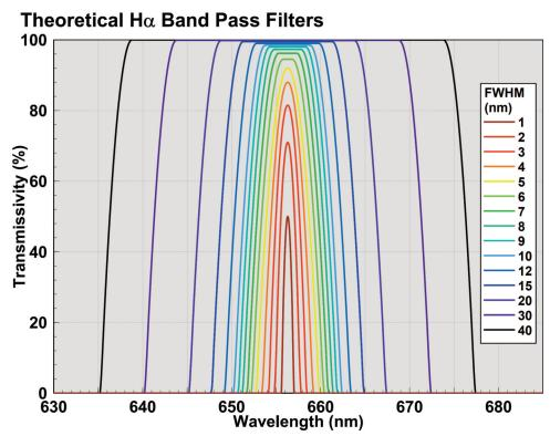
Figure 1 - Spectral Response of Generic H-alpha Narrowband Filters
