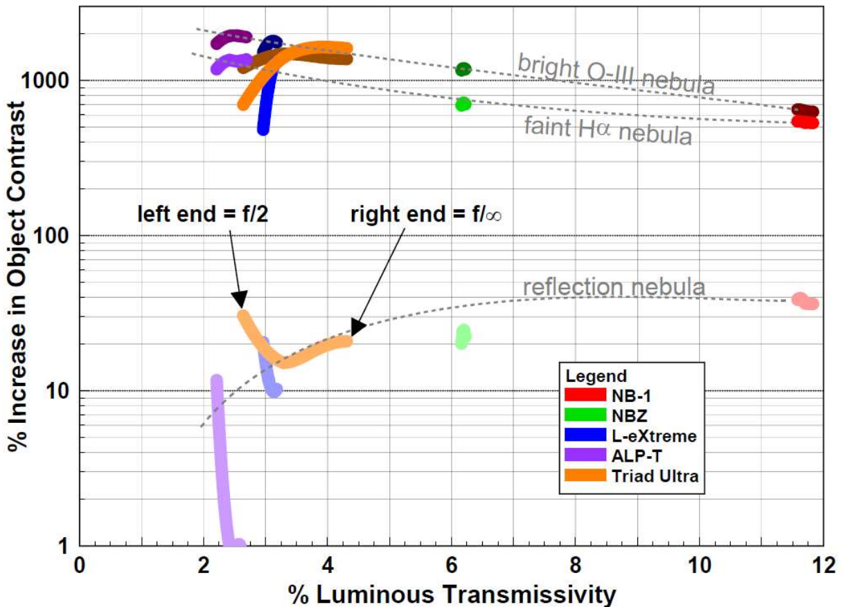
Figure 9 Predicted Filter Performance: Back Illuminated Colour CMOS, LP w/LED (NELM+2.9)
