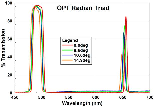
Figure 11 Impact of Filter Angle On Spectral Response – OPT Radian Triad
