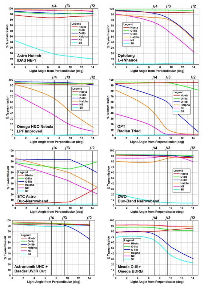
Figure 12 Summary of Angle Impact On Filter Transmission
