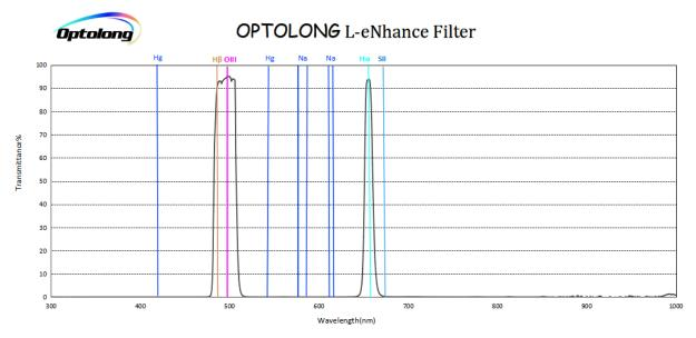
Figure 1 Spectral Response of Example Multi-Narrowband Filter
