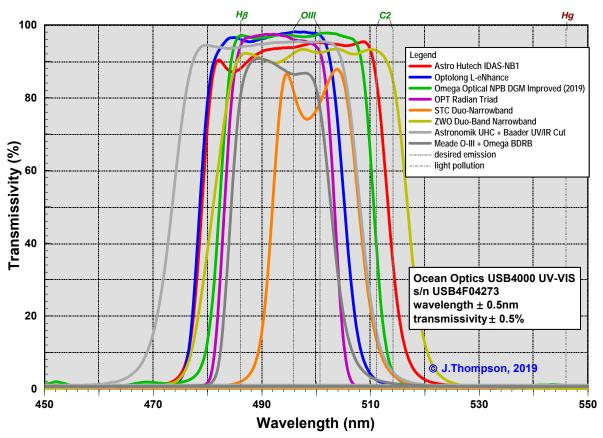
Figure 4 Measured Spectral Response Comparison – O-III Pass Band
