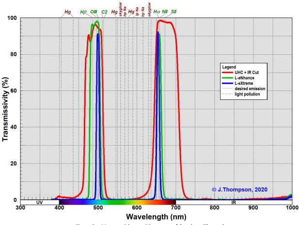
Figure 3 Measured Spectral Response of Optolong Filters - 2
