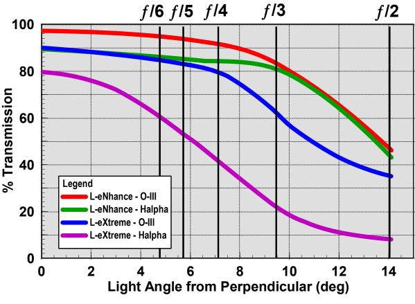
Figure 12 Impact of Angle On Filter Performance
