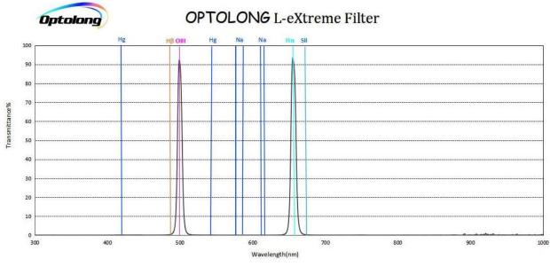
Figure 1 Spectral Response of the New L-eXtreme Filter
