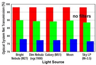
Figure 2. Predicted Optical System Net Transmission – Visual Use: The improvement in image brightness between standard coatings, UHTC coatings, and dielectric coatings is consistent regardless of the target when the scopes are being used visually.
