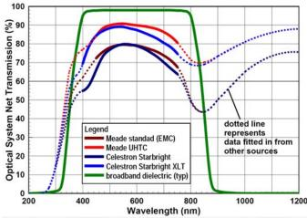
Figure 1. Optical System Spectral Transmission By Coating System: Total system response data is available from Meade & Celestron for the visual band. Data for outside the visual band, and for a typical dielectric mirror has been estimated by combining data from several third party sources.
