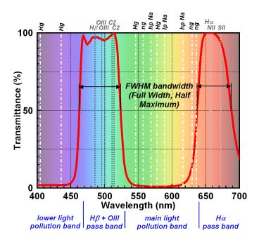
**Figure 2.** Example Spectral Transmissivity Plot: Deep-sky filters tend to have similar appearance as they are trying to achieve the same goal, pass the desirable  $H\beta$ +OIII & Ha passbands, and cut the undesirable light pollution bands. Note that "bandwidth" is normally defined at half the maximum transmittance value of the filter, known as FWHM.
