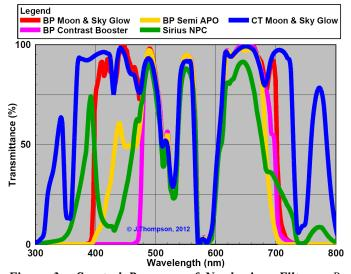
Figure 3. Spectral Response of Neodymium Filters: By infusing the filter glass media with the rare earth element neodymium, a unique and useful family of filters was created.
