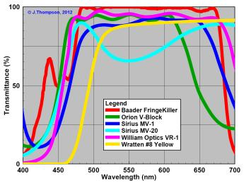
*Figure 4. Spectral Response of Correction Filters: This group of filters is meant for removing the violet-blue end of the spectrum, greatly reducing the appearance of chromatic aberration in achromatic refractors.*
