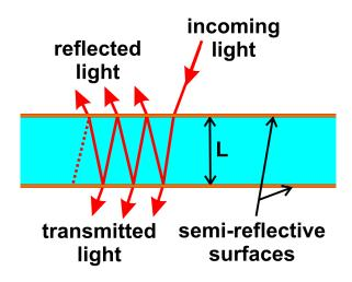
Figure 6. The Etalon: Simply two parallel semi-reflective surfaces, wave interference of the internal reflections allowing only a particular wavelength to pass through. The distance between surfaces adjusts the pass band's centre wavelength, the reflectivity of the surfaces adjusts the pass band's width.
