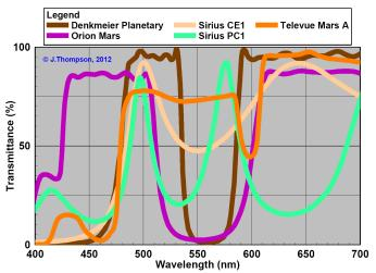
*Figure 2. Spectral Response of Special Planetary Filters: Interference coating technology has been used to make filters that improve the contrast of planetary surface features.*
